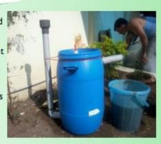
vert organic waste into methane gas through the process of anaerobic digestion.
