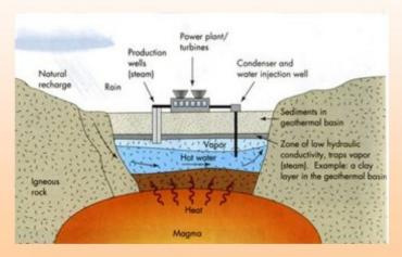
Conditions necessary for a viable geothermal resource include: water, permeability, and heat. These three components create a geothermal reservoir. Geothermal power plants convert the hot water trapped in the reservoir into steam which drives the turbines inside the plant to generate electricity.
