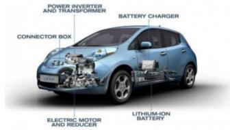
Like other electric and hybrid-electric vehicles, EVs minimize wasted energy by turning the car off when stopped (idle-off) and by charging the battery when braking (regenerative braking).
