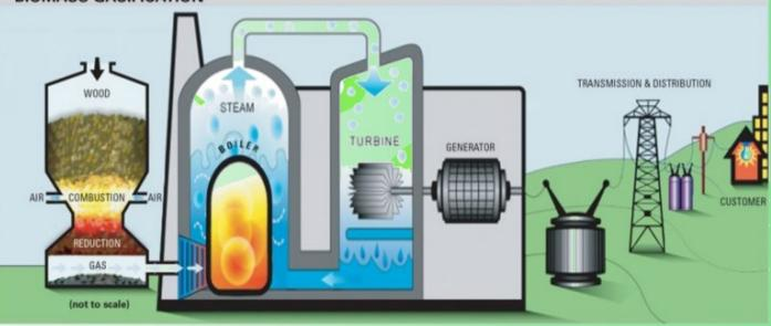
The biomass is collected and processed into a form that can be used at the power plant. It can even be turned into a gas, a process known as gasification.
