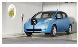
An EVSE is a "home charger" or "wall charger" or "home charging station." It brings AC power to your car, where it is then turned into DC power and charges your car's battery — via the car's onboard charger.
