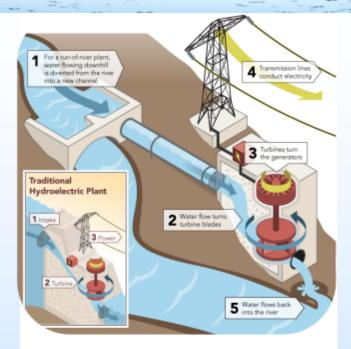
To harness energy from flowing water, the river is dammed to create a reservoir. Water is channelled through tunnels in the dam. The energy of water flowing through the dam's tunnels causes turbines to turn. The turbines make generators move thereby producing electricity.
