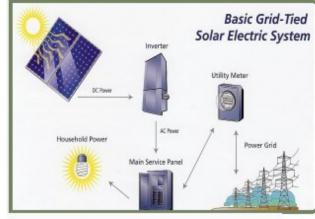
Basic Grid-Tied Grid Tied Systems allow you to utilize both the solar power and the utility's power at the same time. It also provides the opportunity to sell any excess power produced by the solar system
