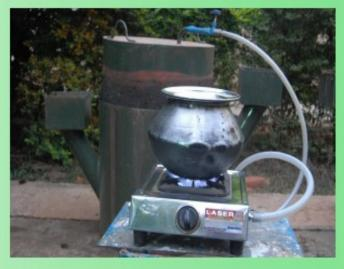
The methane gas produced may be used for cooking, lighting, and other energy needs. Waste that has been fully digested exits the system in the form of organic fertilisers.
